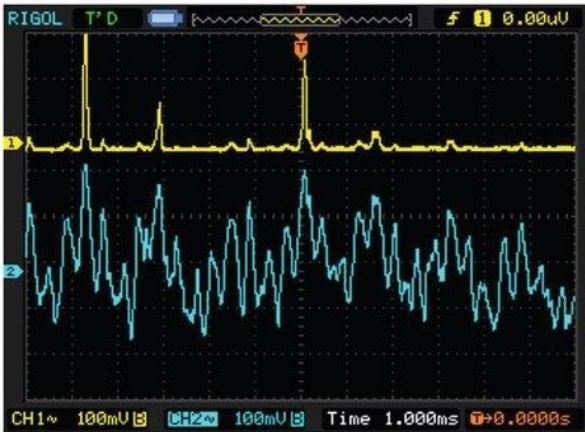
Oscilloscope trace showing the bad channel. Trace (1) showing the output of the defective side — only responding to high peaks and only in the positive direction, while trace (2) shows the other channel's correct output.
